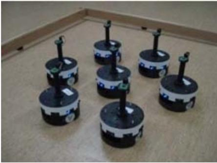
FIG. 39 (Color online) A photo of seven mobile robots (called “Kobots”) moving in a swarm. According to Turgut *et al.* (2008), the main factor defining the size of the swarm (the number of Kobots flocking together) is the range of communication, and it is highly independent from both the noise (encumbering the sensing systems) and from the number of neighbors each robot had. Adapted from Turgut *et al.* (2008).
